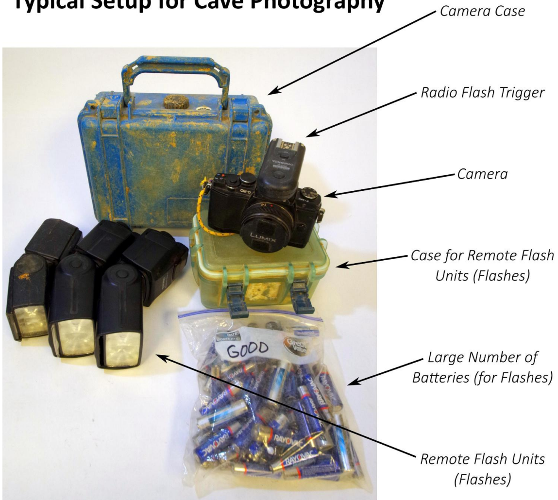
Figure 5. The standard setup for cave photography. This same setup is used to create photogrammetry model/maps of cave features/passages.
