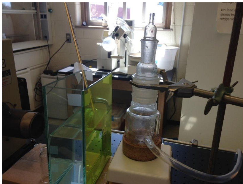
Figure 14. Close up of the water filter and the uncapped photoreactor. It is capped with a septum during runs.
