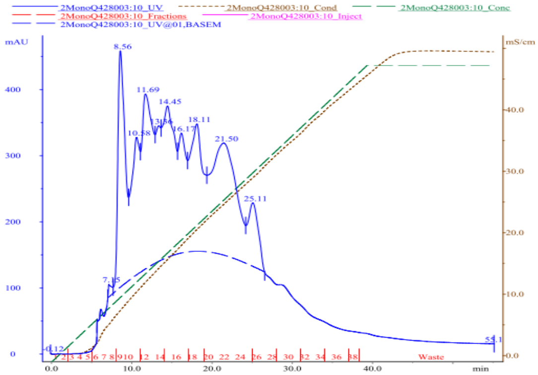
Figure 15: Chromatography profile of protein in Mono Q column purification. The absorbance of protein at 280nm (blue line), salt conductivity (brown line), and collected fraction (0.5ml) (red line). Fractions #15-51 were used for SDS gel and western blot analysis.
