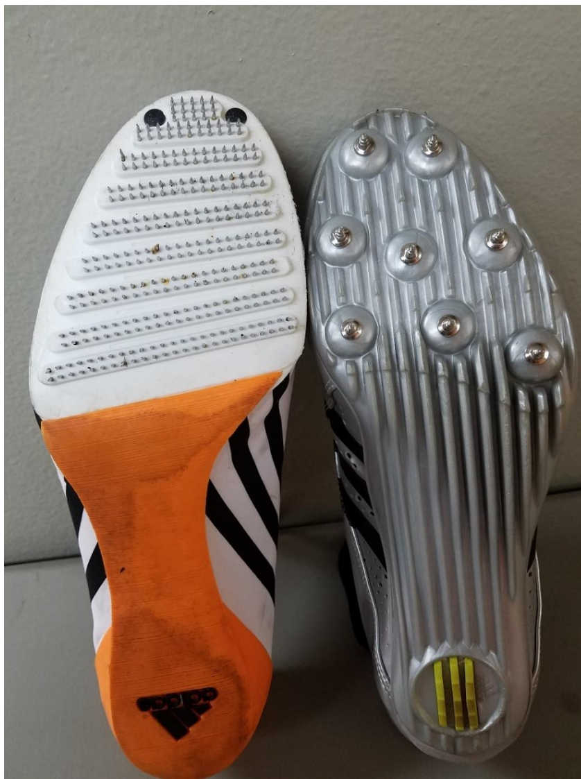
Figure 2.2. Comparison of the ground and ice contact surface and spike design of bobsled brush spikes with track and field sprint spikes.
