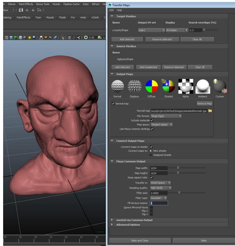
(Fig 14. Setting up the Envelope of the low poly mesh to read the detail of the high poly mesh in Maya.)
