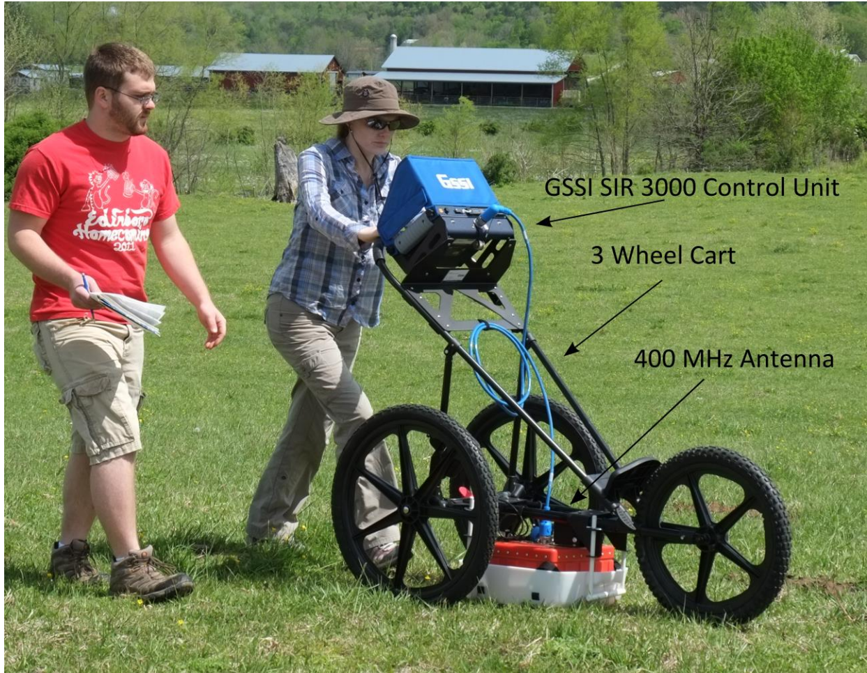
Figure 19. GPR Cart System. GSSI SIR 3000 control unit with three wheel cart and 400 MHz antenna. Photographed 05/02/2014.
