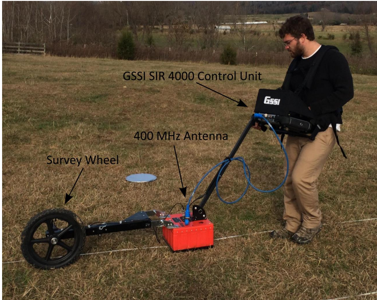
Figure 13. GPR System. Geophysical Survey Systems Inc. (GSSI) SIR 4000 control unit paired with a 400 MHz antenna and a survey wheel.
