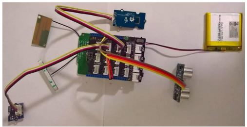
Fig. 5-5: Li-Po battery added
