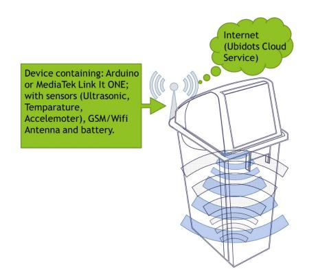
Fig 1-3: The Eco-Smart Can concept.
