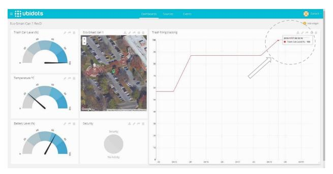
Fig. 9-5: Ubidots dashboard- Trash full (100%)
