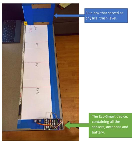
Fig. 9-1: Device testing system.
