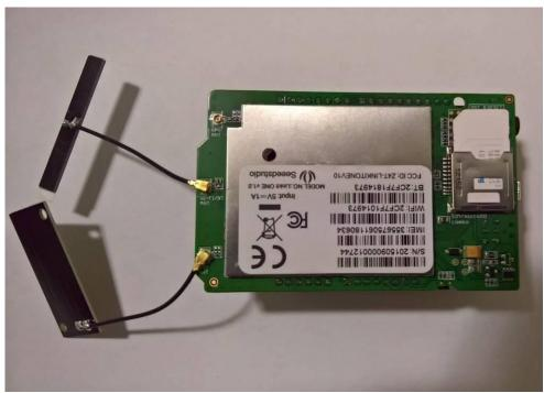
Fig. 5-1: GPRS & Wi-Fi antenna & Ting 2G Sim card.
