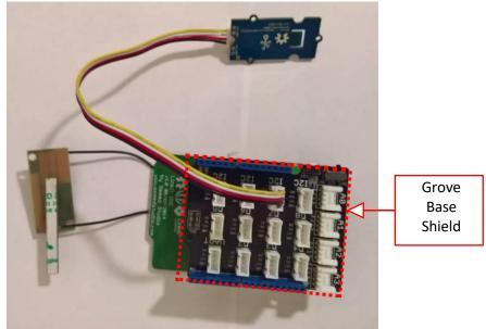
Fig. 5-2: Temperature & Humidity sensor
