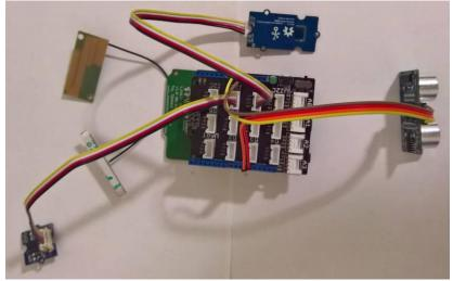
Fig. 5-4: Ultrasonic sensor (HC-SR04)
