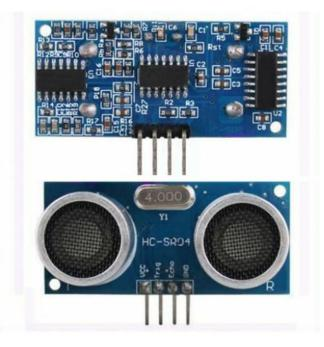
VCC = +5VDC Trig = Trigger input of Sensor Echo = Echo output of Sensor GND = GND
