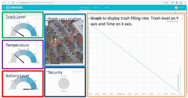
Fig. 9-3: Ubidots cloud service Dashboard
