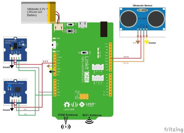
Fig. 4-1: Board connection layout (Developed with Fritzing Software)
