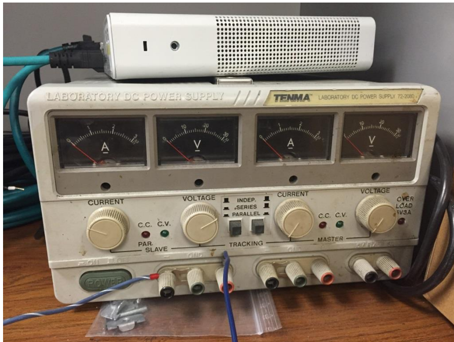
Figure 6: Tenma 72-2080 DC Power Supply
