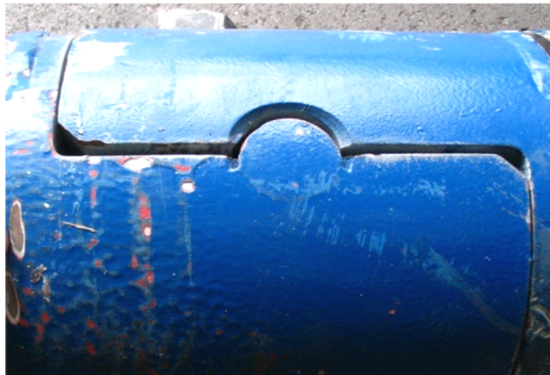
Figure 2. A Track Coupling is Shown, Consisting of Two Major Steel Castings and Similar to the Type Evaluated during the Study
