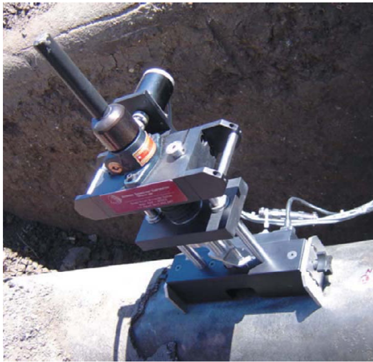
Figure 8. SSM System Mounted on a Section of Steel Gas Pipeline Using Magnetic Mounts
