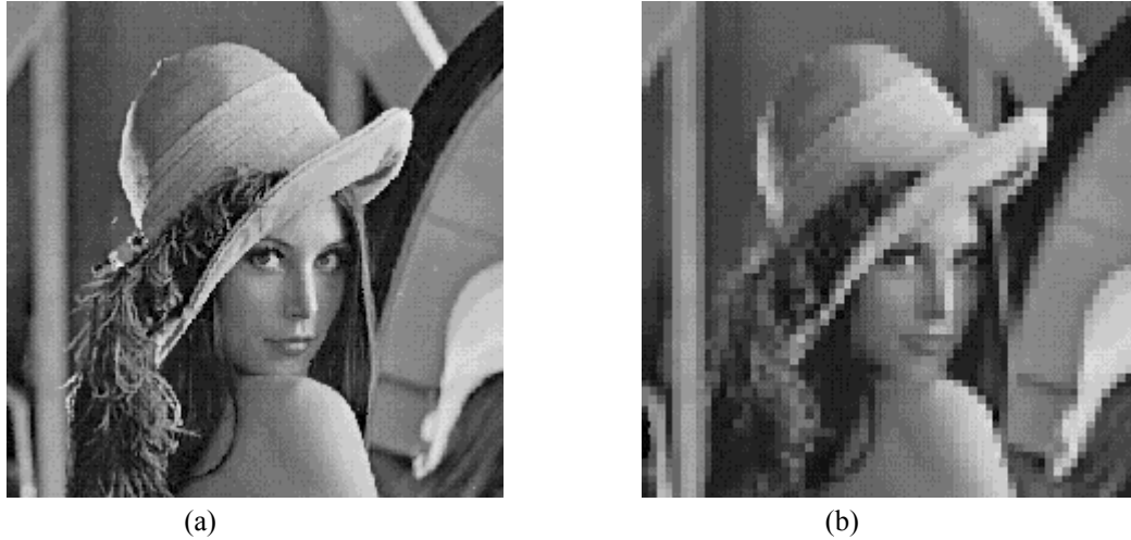
Figure 5. (a) Original Lena Image (b) Reconstructed image to show blocking artifacts
