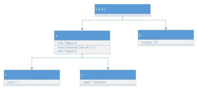
Figure 15 - Composite object to be written to JSON
