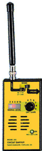
Figure 7. Selected E-Field Detection Unit for Arc Detection System
