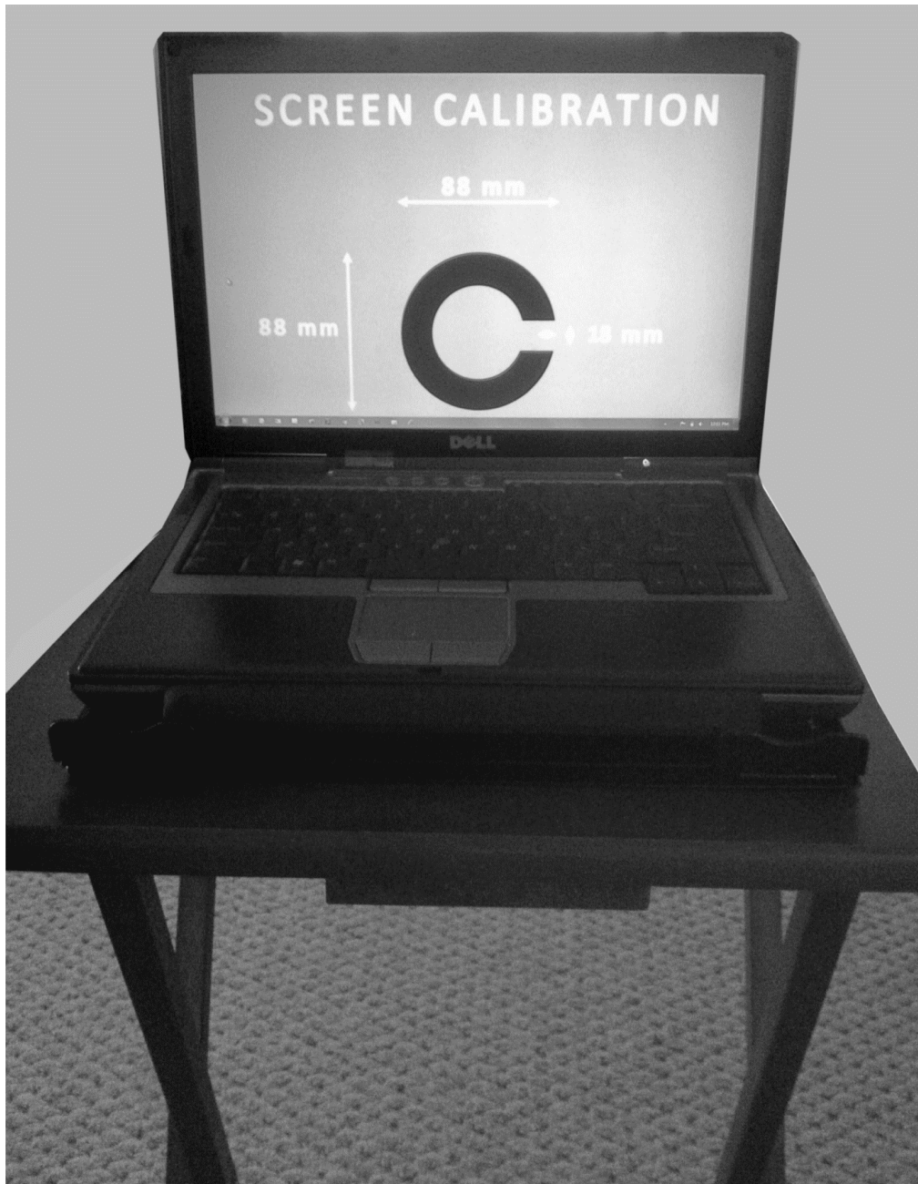
Figure 44. Display Setup Using the Calibrated C Optotype
