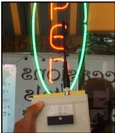
Figure 11. False positive (caused by the switch-mode power supply for a neon sign) is detected by the early laboratory development detector
