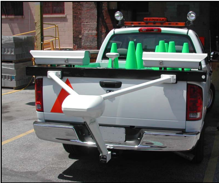
Figure 2. Mobile (truck-carried) scanner
