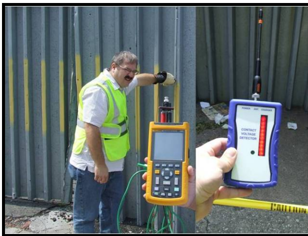
Figure 18. Energized fence caused by energized earth detected by a beta detector
