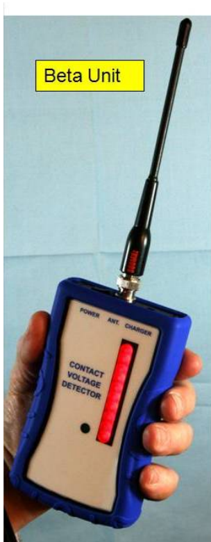
Figure 4. Beta version of handheld emissions detector
