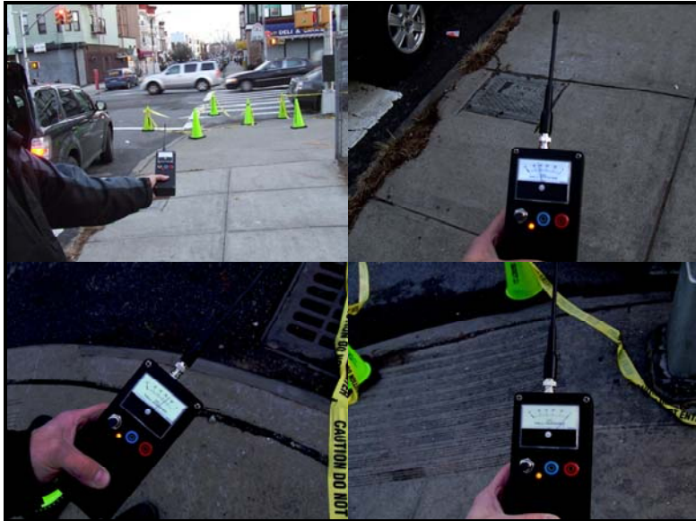
Figure 13. Demonstration of increasing signal strength as an energized object is approached by an alpha unit–generation 1
