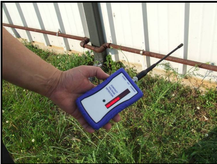
Figure 16. Detection of induction coupling between an overhead power line and gas line
