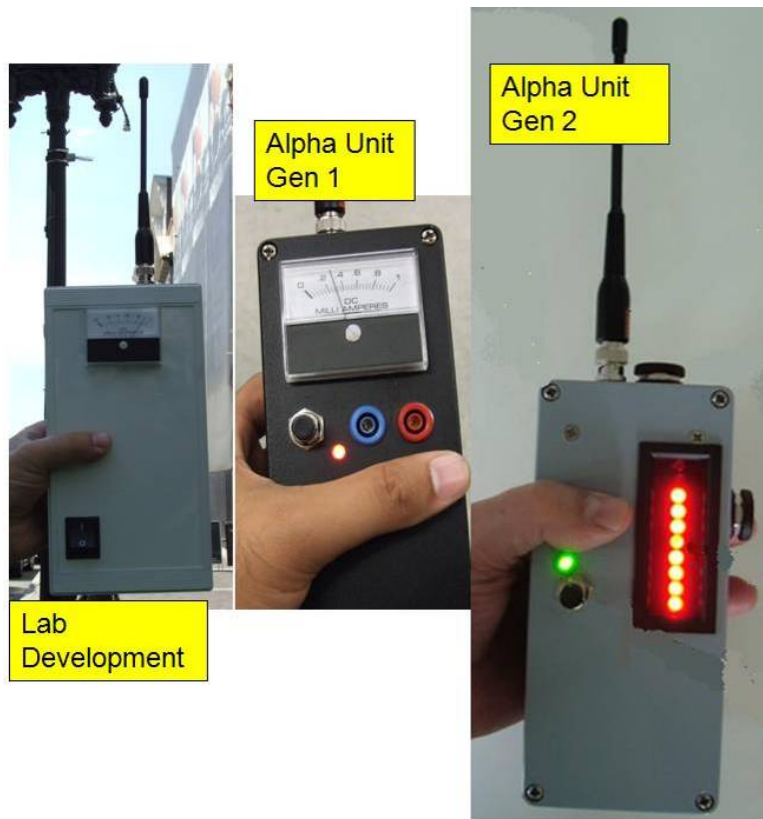
Figure 3. Chronological development of the new handheld detector
