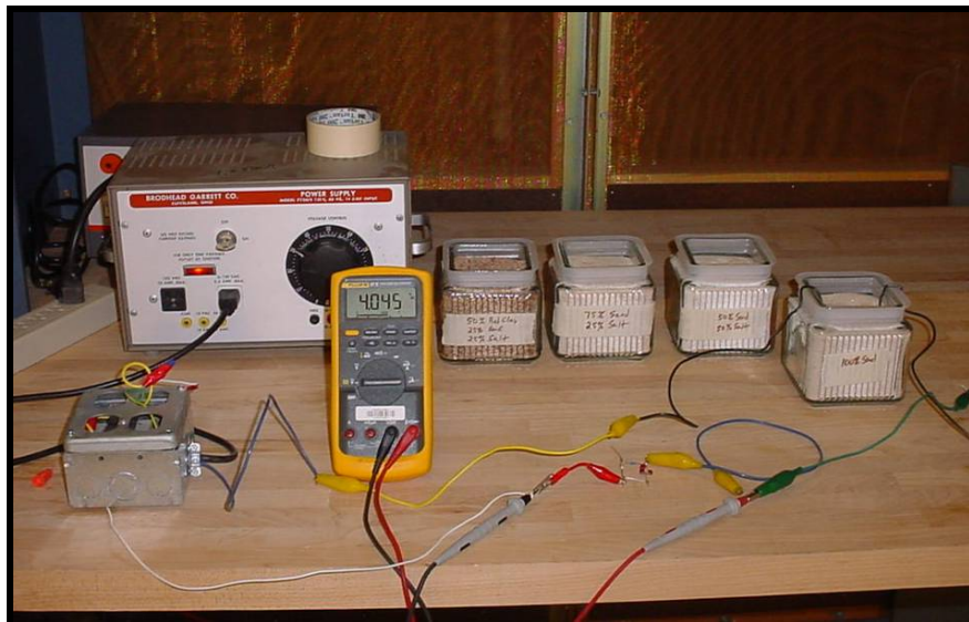
Figure A-4. Test Setup—Showing Variac, Fluke voltmeter, transformer, and samples of four soil mixtures
