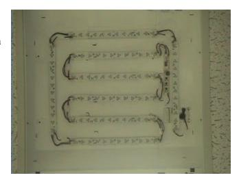
*Figure 4*. Installation of LED Light Bars, Concept 3b
