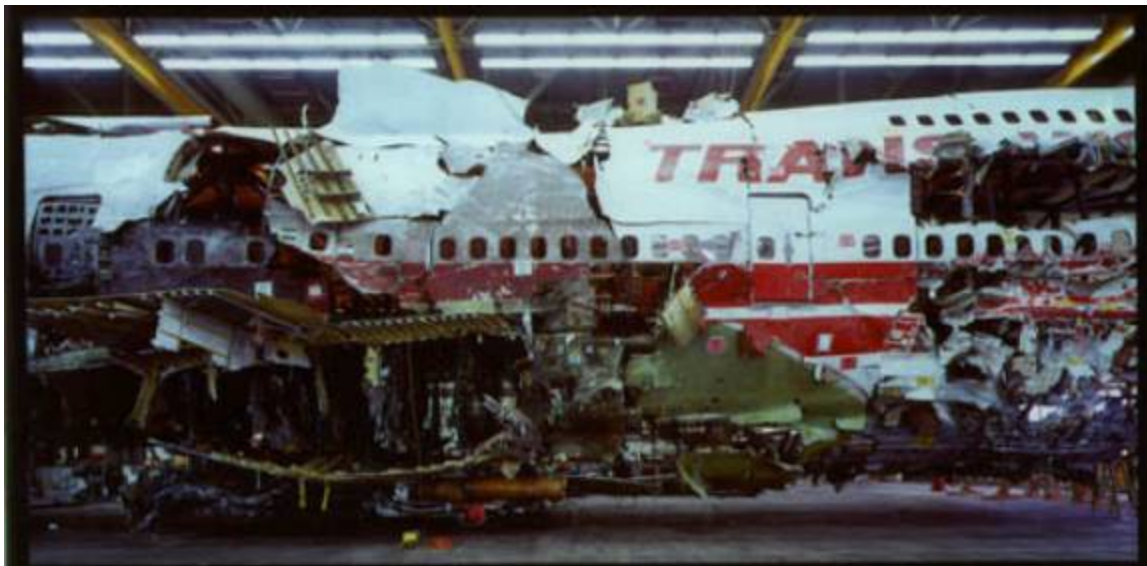
Figure 1. TWA Flight 800: The Reconstruction (1999).
