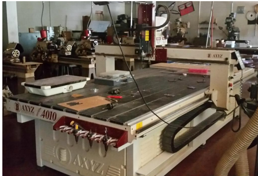
Figure 7. XYZ 4010 CNC Router
