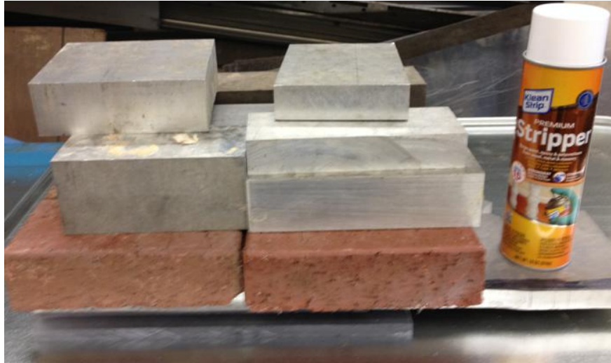
Figure 29. Pressed Bonding with Klean Strip®
