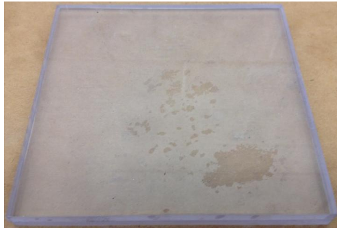
Figure 17. Resulting Air Pockets (30 Minutes at 180°F)
