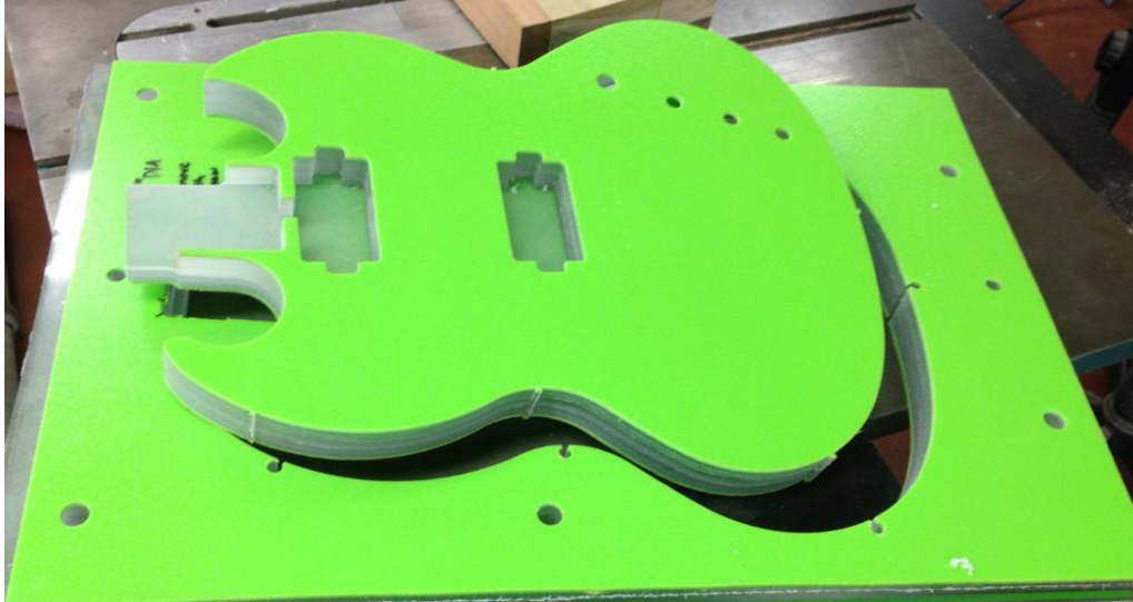
Figure 63. Removal of the Laminated Guitar Body
