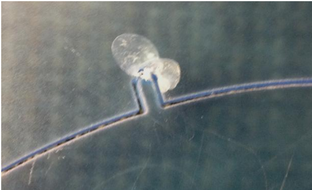
Figure 46. Example of Waterjet-Induced Bottom Blowout of 1/4" Tab
