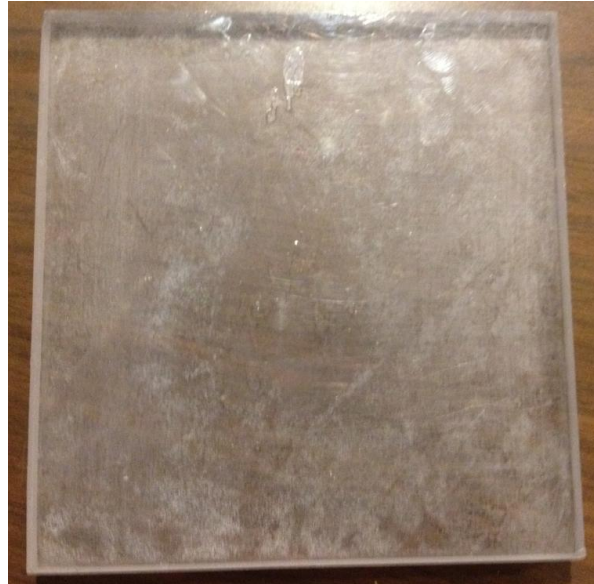
Figure 28. MEK-Saoked Sponge Brush Experiment 6" x 6" Nom. 1/4" (6mm) Specimen
