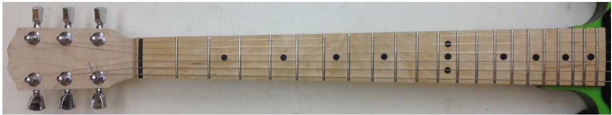
Figure 70. Modified Guitarbuilding.org Maple Neck with Custom Maple Fretboard
