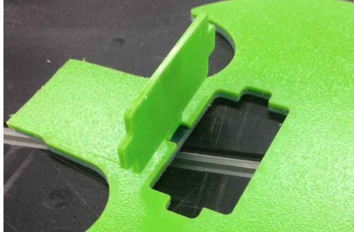
Figure 54. Example of Undesired Neck Pocket Bonding
