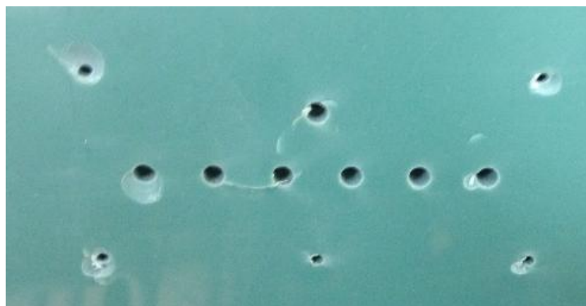
Figure 43. Example of Waterjet-Induced Blowout on Bottom Surface
