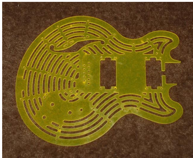
Figure 1. First Proof-of-Principle "Space Frame" Copolyester Guitar
