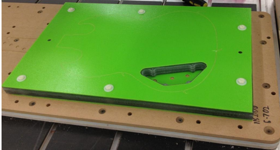
Figure 37. Copolyester Body Blank Mounted on XYZ Guitar Tooling
