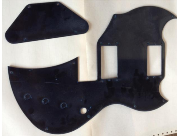
Figure 67. Faceplate-Pickguard and Cavity Cover Laser-cut from 2mm Black Copolyester
