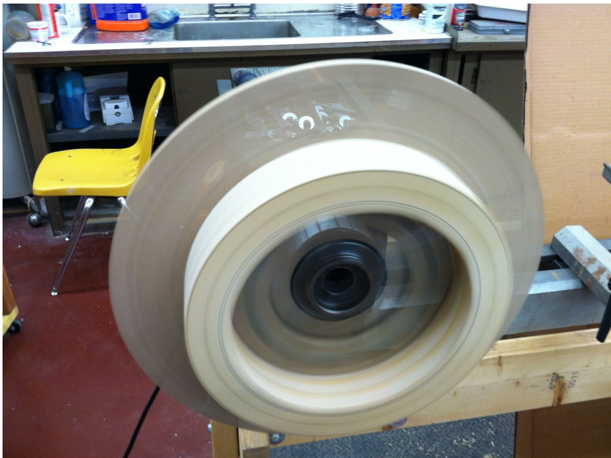
Figure 9. Block Rim Being Turned. After modifying the Cole adapter set to accept the rim, the rim was able to be held securely by the extensions and turned to final shape using hand tools.
