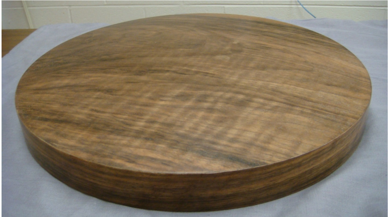
Figure 21. Resonator after Finishing. The third resonator after walnut veneer was applied and finished with Truoil.
