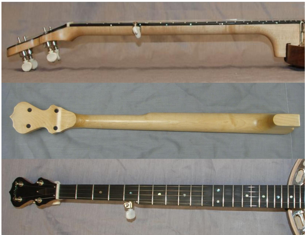
Figure 23. Top, Side, and bottom View of Finished Neck. The finished maple neck is shown after a coat of Truoil was applied.
