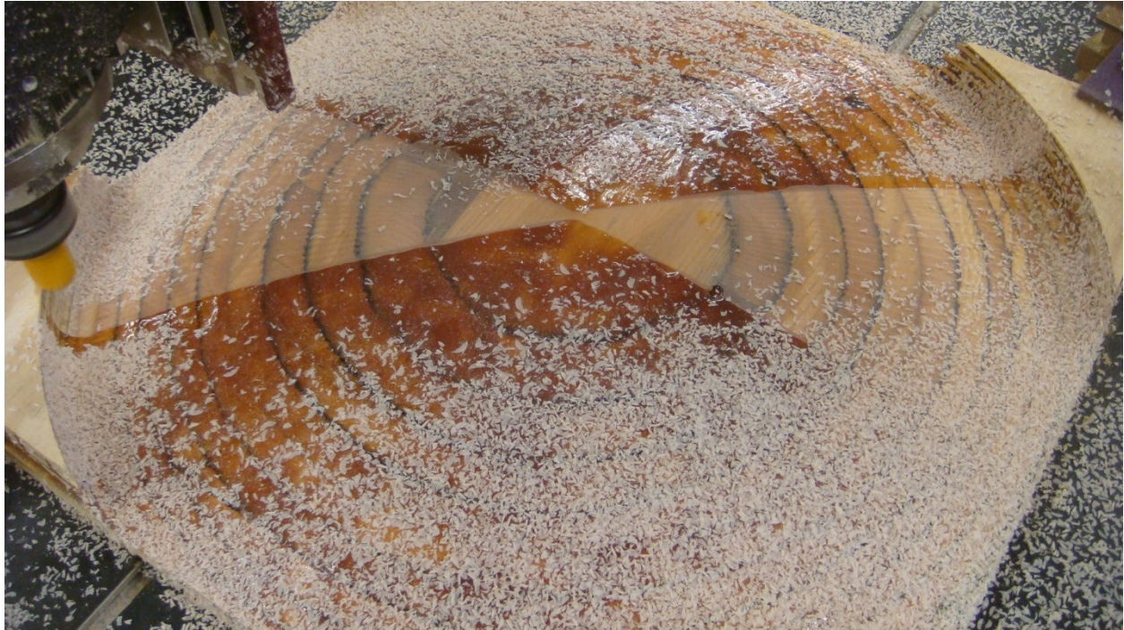
Figure 2. Cutting the Convex Epoxy Surface. The convex surface was cut a second time after a coat of epoxy filled in some areas due to voids within the internal laminations.
