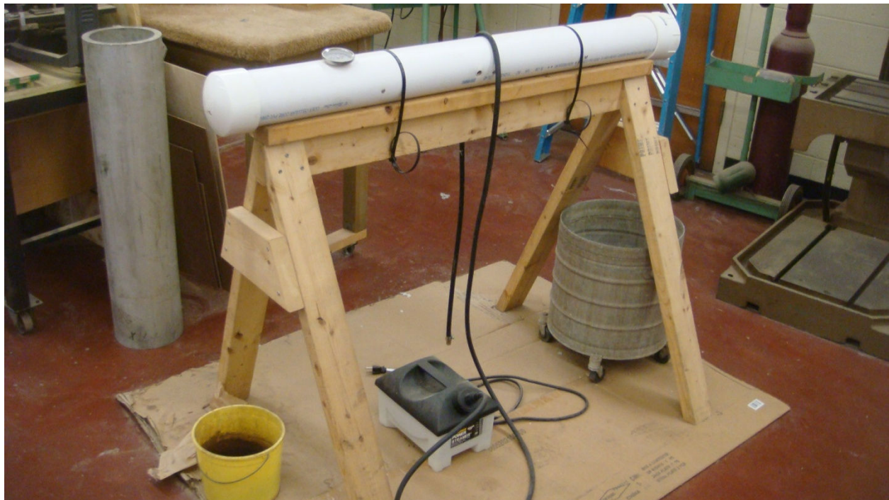
Figure 4. A Look at the Steam Chamber. The steam chamber softened the wood strips so the pliable strips could be bent to be bent.
