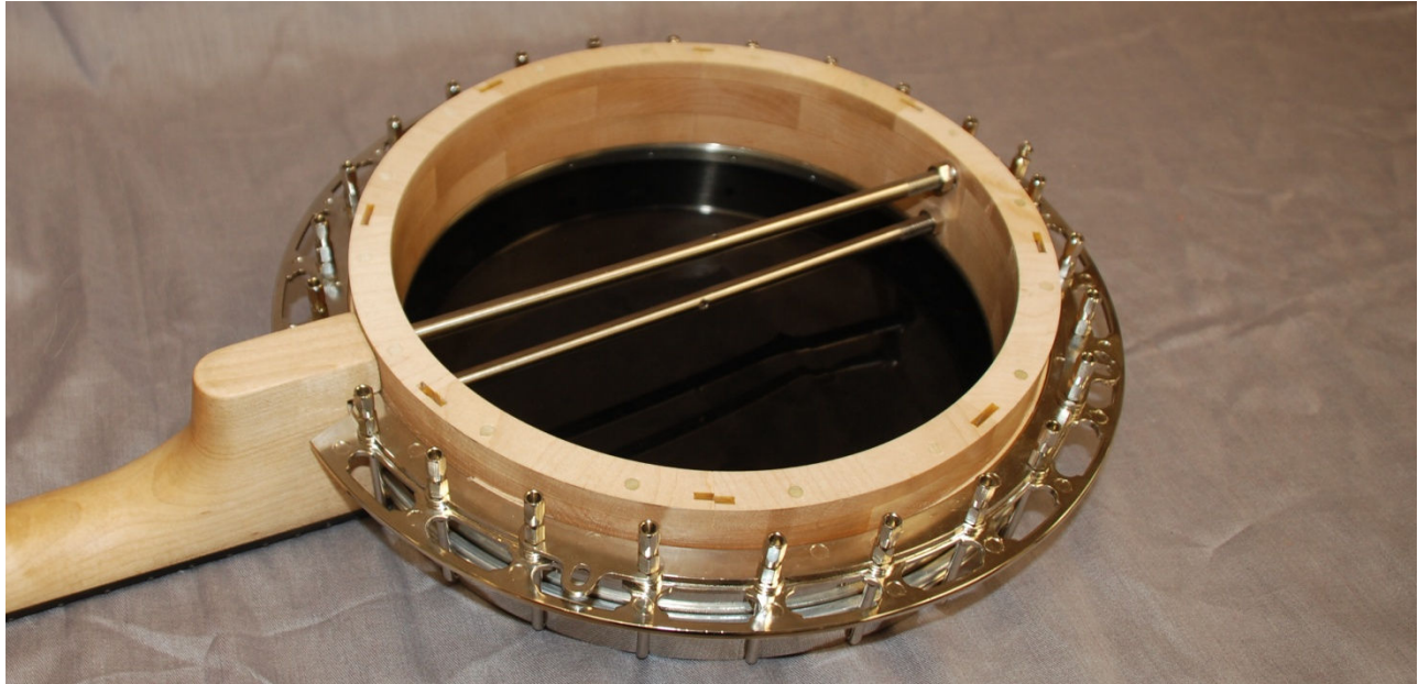
Figure 22. Assembled Rim and Pot Assembly. The rim after pot assembly and the neck was installed.
