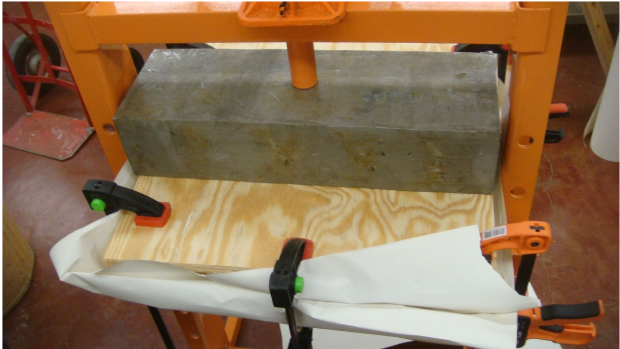
Figure 3. Using the Matching Radiused Forms. The 1/4" plywood material was pressed between the matched press forms for shaping.
