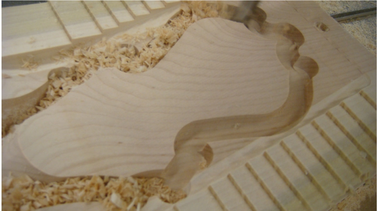
Figure 17. Headstock Cutout Tool Path. Redesigned headstock followed traditional banjo headstock designs.
