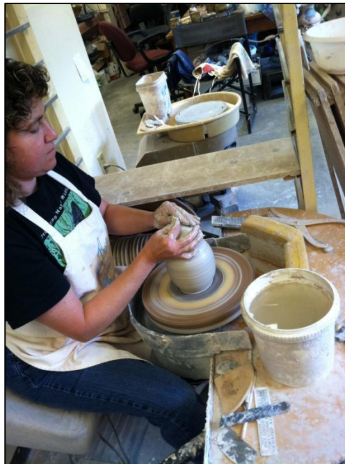
{Figure 15} After throwing a cylinder form, Buie brings the walls in to close the top of the jar.
