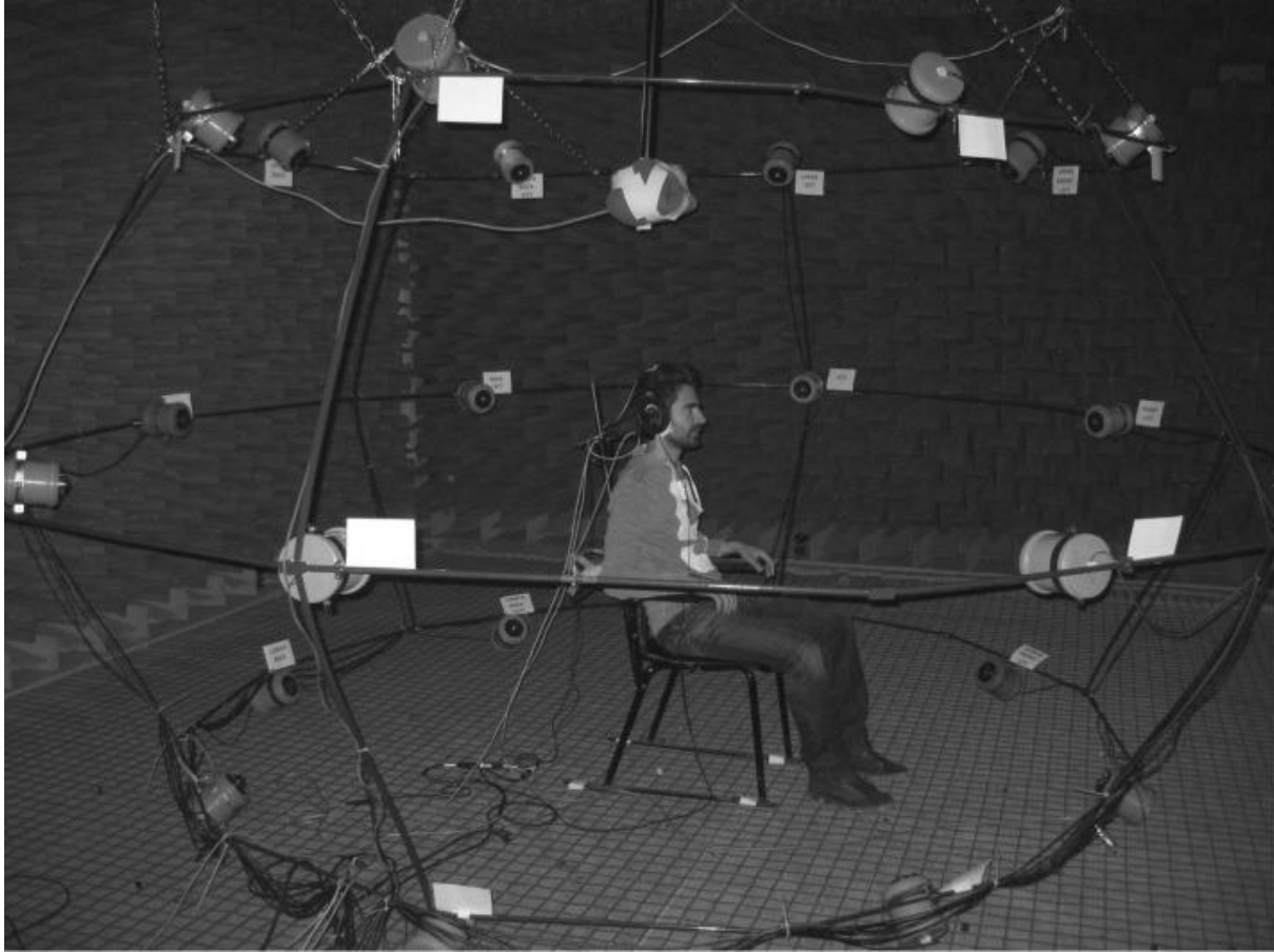
Figure 20. 5.1 Anechoic room with loudspeaker setup and subject. Experiments on Authenticity and Plausibility of Binaural Reproduction via Headphones Employing Different Recording Methods
