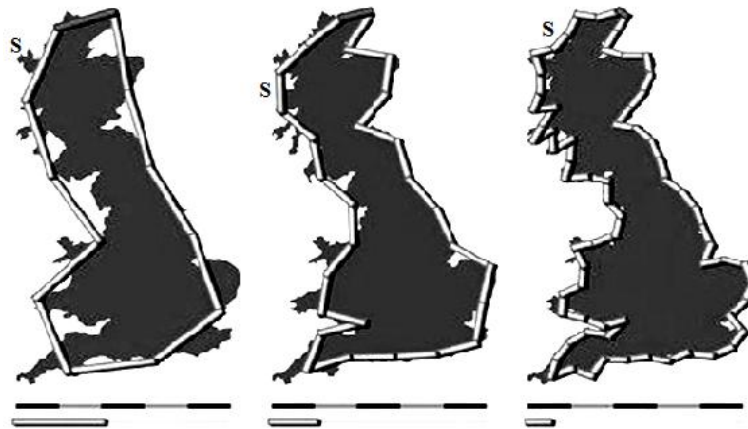
Figure A. 1. Measurement of the British coastline with different yardsticks ( S ) leads to different lengths ( L ). http://commons.wikimedia.org/wiki/File:Britain-fractal-coastline-combined.jpg
