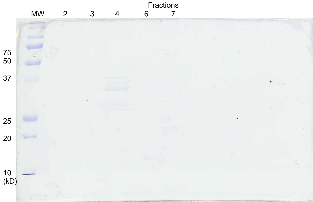
Figure 13: SDS-PAGE of fractions 2, 3, 4, 6, and 7 from Figure 12. The first lane (MW) contains the Precision Plus Protein® molecular weight marker standard. Fraction 4 shows three protein bands, one at approximately 35 kD, another at 33 kD and one at 30 kD. The other lanes contain no visible protein.
