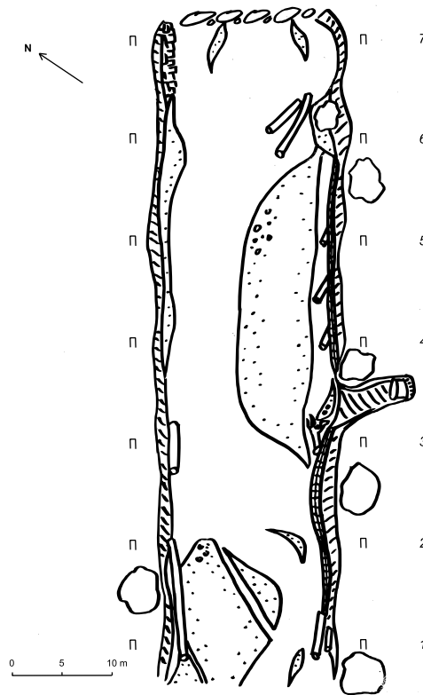
Figure 3.4 – North Experimental Site sketch Interpretation of the NES channel with locations of cross-section transects numbered in the upstream direction.
