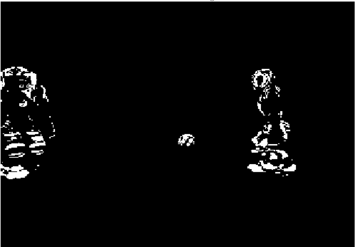
Figure 8.2: This is an example of a sequential scene used to test binary thresholding. Note that both the robots and the ball are moving.
