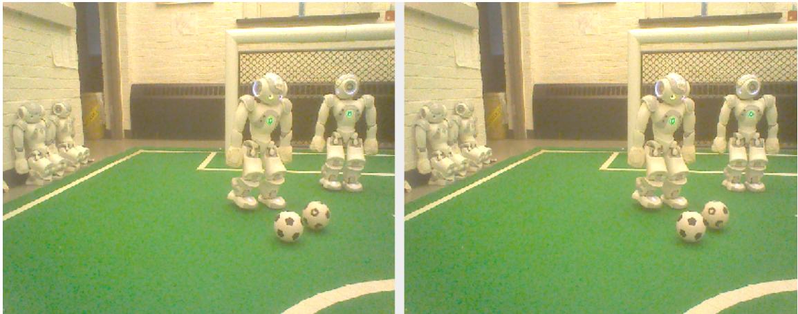
Figure 6.1: This is an example of a sequential scene used to test the absolute differential method. Note that everything in the image except the leftmost ball is moving.
