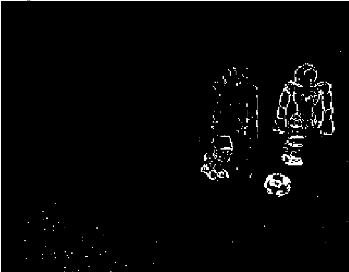
Figure 6.1: This is an example of a sequential scene used to test the absolute differential method. Note that everything in the image except the leftmost ball is moving.
