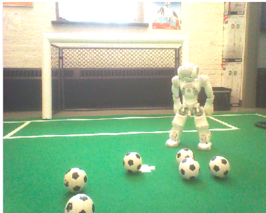
Figure 8.6: This is an example of an image used to test the binary threshold with natural or extreme lighting.
