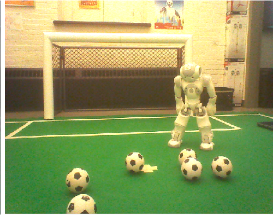
Figure 8.5: This image is an example of an image used to test the binary threshold with average lighting.
