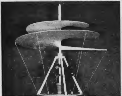
Shown above is a scale model of a design for an aerial screw, resembling the helicopter of the present day, and also credited by many as being the forerunner of the modern propeller. (Model of invention by Leonardo da Vinci.)
