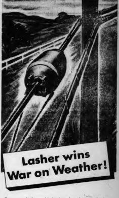
For years, telephone cable has been hung by stiff wire rings from its supporting strand. But repeated expansion and con-traction caused by temperature changes sometimes proved too much-for even the best cable sheath. Fatigue cracks
