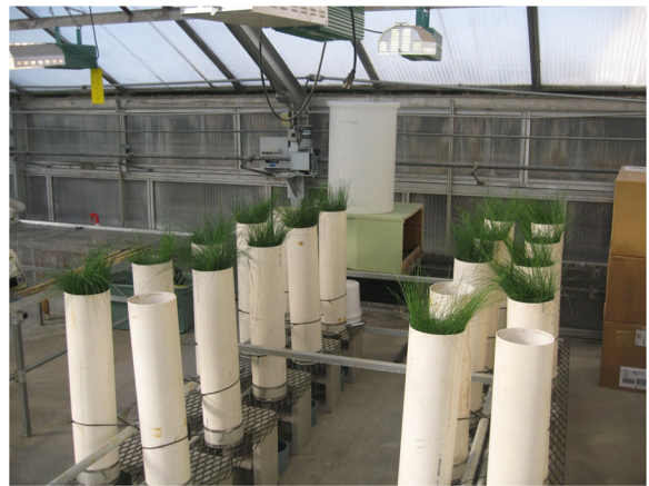
Fig. 1 Columns supported 40 cm off the ground using rustproof-painted metal support gratings and concrete blocks
