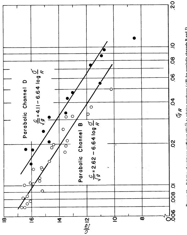
FIGURE 19.—Relation of resistance coefficient  $(C/\sqrt{q})$  to relative roughness  $(\sigma/R)$  for parabolic channels B and D.
