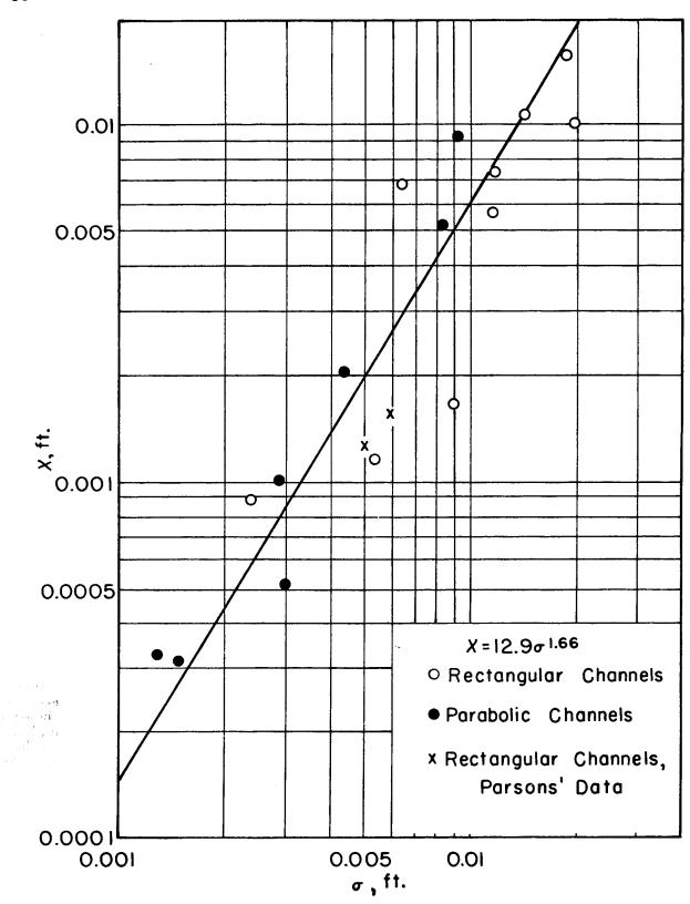
FIGURE 24.—Relationship of resistance parameter, x, to roughness height,  $\sigma$ .
