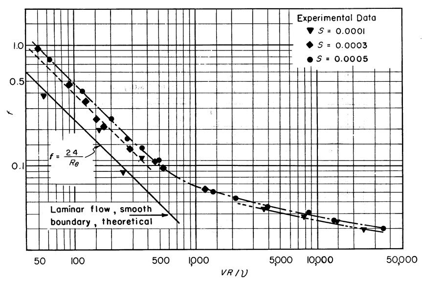
FIGURE 7.—Resistance coefficient f as a function of Reynolds number,  $VR/\nu$ , for rectangular channel K.
