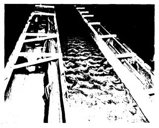
FIGURE 28.—Rectangular channel F. A large, erosive stream of water was used to form relatively large ripples.
