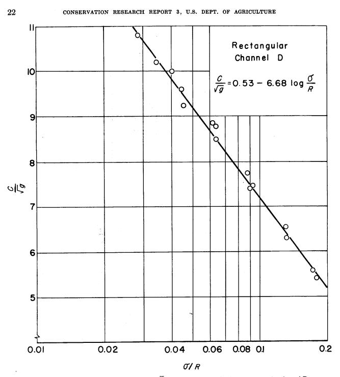
FIGURE 13.—Relation of resistance coefficient  $(C/\sqrt{g})$  to relative roughness  $(\sigma/R)$  for rectangular channel D.
