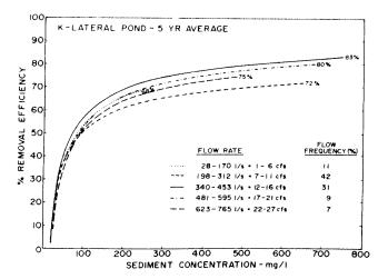
FIG. 3 The effect of sediment concentration and flow rate on the sediment removal efficiency.
