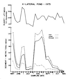
FIG. 2 Surface water runoff and sediment entering, retained, and leaving the sediment pond during the 1975 irrigation season.
