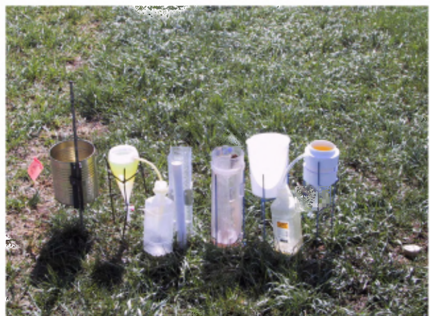
Figure 2. Catch-cans in the field, from left to right: metal can, separatory funnel, wedge rain gauge, funnel rain gauge, white bucket, and PVC reducer.
