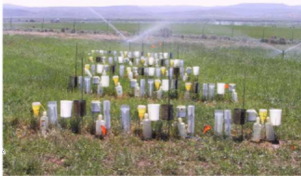
Figure 6. Catch-can setup in the field from I1 (nearest row of catch-cans) to I5 (furthest row of cans) with line-source sprinklers in background (Randolph, Utah, 2004).
