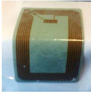
Fig. 2 The attachment of a HF tag on both sides of a product
