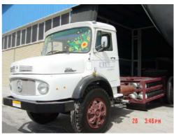
Clearly, for reinforcing the body with purpose of keeping the tanks and preventing concentration of tension in these points (because of increased weight), some modifications has been made on the body, chassis or different parts. In this system, different type tanks have been used side by side. Faber Company and MCS Company have made these tanks of steel or aluminum and reinforced them with composite fibers in radial direction .
