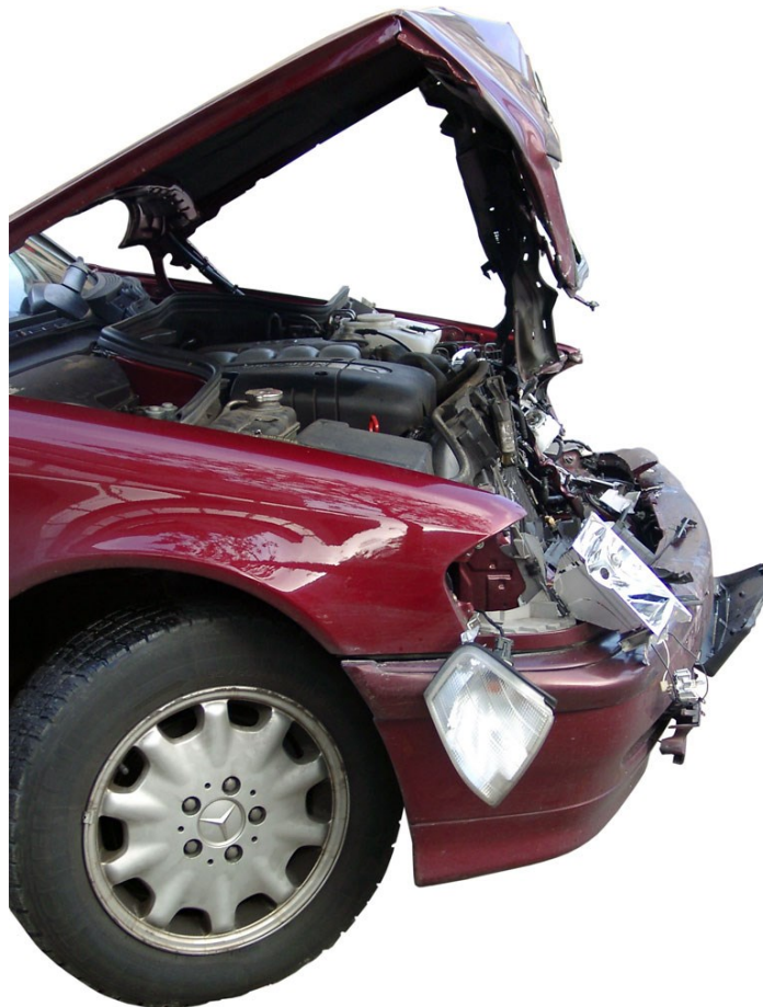
Figure 1: Crumple zone damaged in a car collision. Photography courtesy of Julu [CC-SA 3.0 https://goo.gl/jSL8Ax ].
