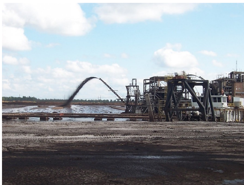
Figure 2: North Maxville Mine - Dredge mining for heavy minerals. Photograph courtesy of Florida Department of Environmental Protection.
