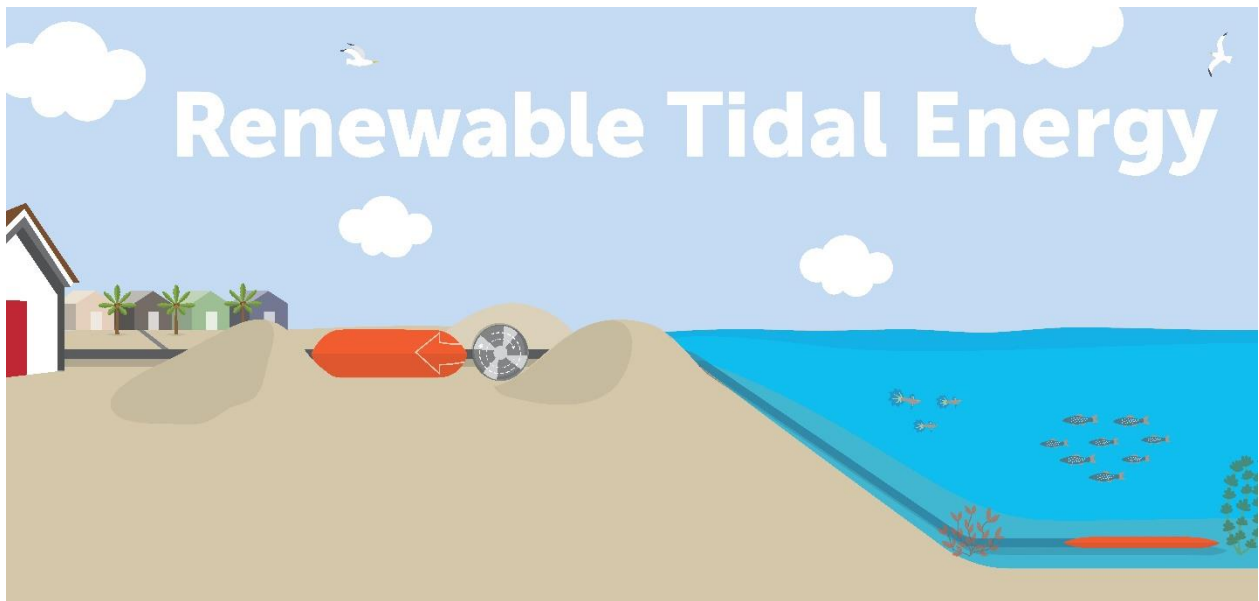
Figure 2: Infographic illustrating the proposed closed convergent tidal system. The closed convergent tidal generator uses two compliant flexible bladders, one offshore and the other offshore to derive energy from the tidal range. The onshore option of generator placement allows for easy of installation and maintenance. The closed system eliminates biofouling and interactions with local ecology.
