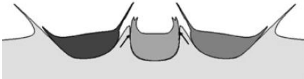
Figure 22. Multi-particle interaction for an impacting velocity of 600 m/s: extrusion effect [37].
