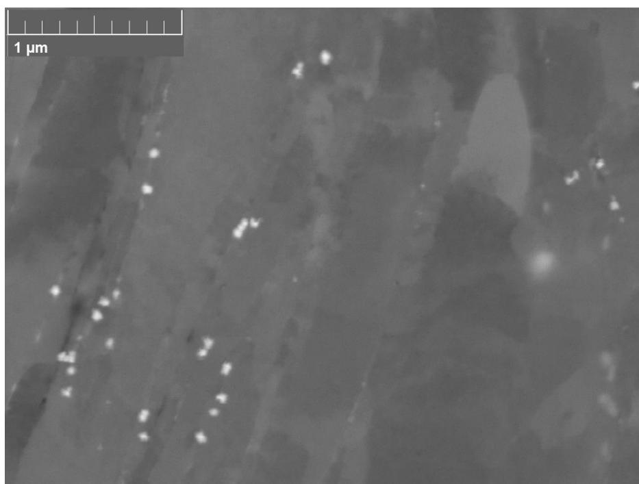
Figure 64. SEM micrograph taken in BSE mode of AR high deformation region.
