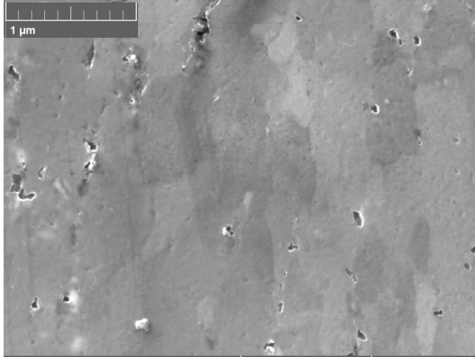
Figure 70. SEM micrograph taken in SE mode of 100 hour high deformation region.
