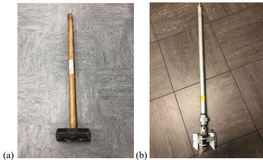
Figure 8. Seismic sources. (a) Seismic source for terrestrial sites. (b) Seismic source for marine sites.
