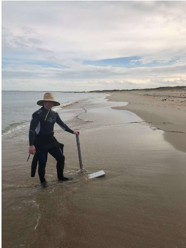
Figure 17. MASW setup at MASW Site #2
