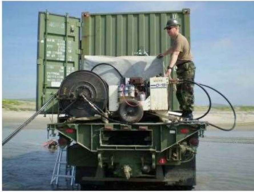
Figure 26. Hydraulic power unit used for RPT operations
