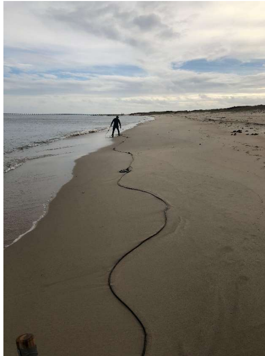
Figure 22. Hydrophone string in sinusoidal configuration in surfzone
