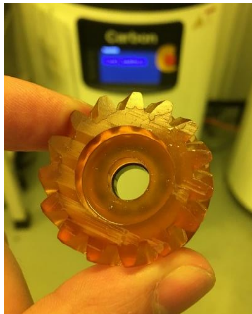
Figure 19 - 3D Printed Custom Idler Pulley via Carbon M1
