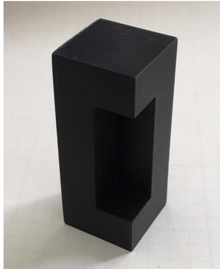
Figure 37 - Coupon used to calibrate mechanical actuation of the sensor
