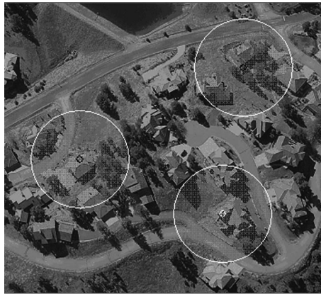
Figure 1 - 5 GHz: Bandwidth is good but measured range (circle) is poor. Range is not sufficient to bootstrap mesh until installed percentage is quite high (in this diagram ~50%)
