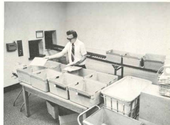
These four Phillipsburg inserter machines will handle over 11 million pieces of mail this year at Blue Cross and Blue Shield. The machine in the foreground is the newest one purchased which is capable of stuffing inserts up to 9½" X 12½" in size.
