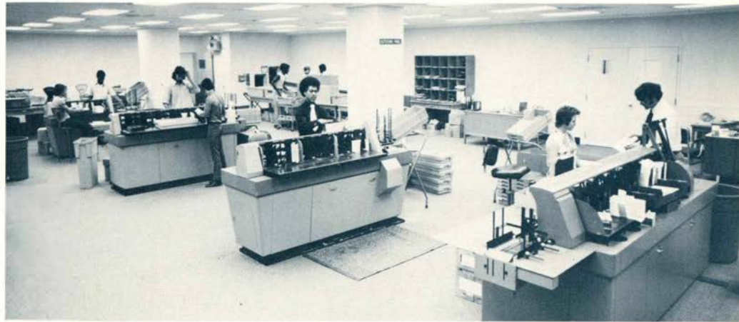
These four Phillipsburg inserter machines will handle over 11 million pieces of mail this year at Blue Cross and Blue Shield. The machine in the foreground is the newest one purchased which is capable of stuffing inserts up to 9½" X 12½" in size.
