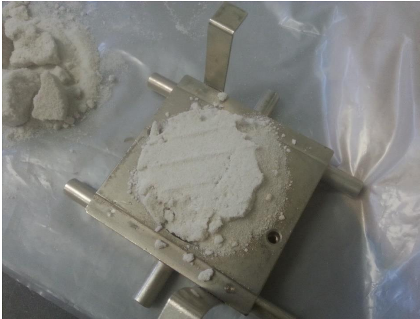
Figure 4-11. Post DST specimen of 2-3" sample
