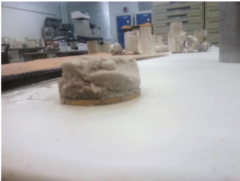
Figure 4-10. Post DST specimen of 1-2" sample
