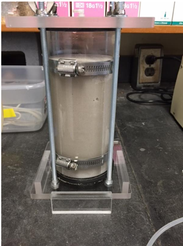
Figure 3-3. UCDM treatment chamber filled with Ottawa 50-70 sand
