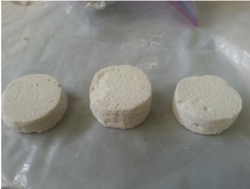
Figure 4-8. DST samples from varied height intervals from the bottom of the specimen
