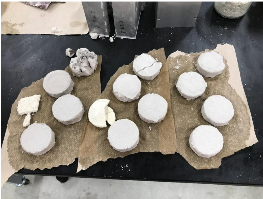
Figure 3-11. Treated SMM sand samples prepared for DST
