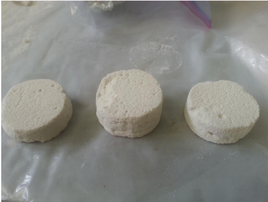
Figure 3-10. Treated UCDM sand samples prepared for DST
