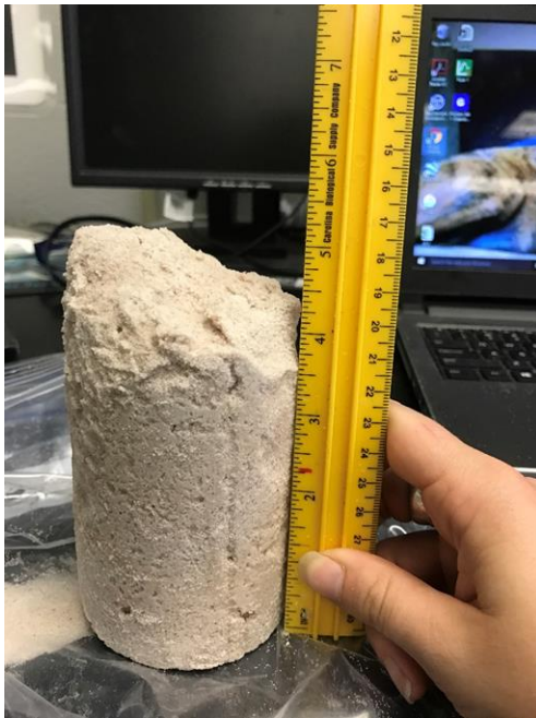
Figure 4-7. Example of full cemented soil column
