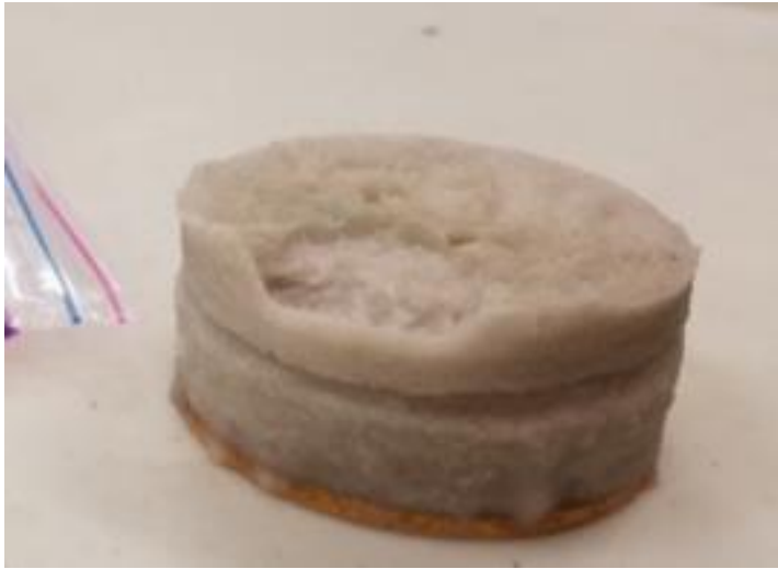
Figure 4-9. Post DST specimen of 0-1" sample
