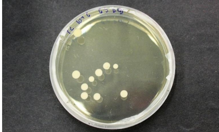
Figure 8. Picture of colony forming unit plate. This CFU plate was made with solid growth medium and a diluted fermentation sample. Each round colony is assumed to arise from a single, viable yeast cell. This plate, then, would indicate ten colonies.
