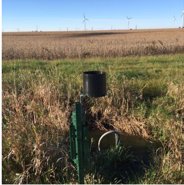
Figure 9. Rain gauge setup used at each site. I attached Rain gauge to the post that houses the logging end of the pressure transducer.
