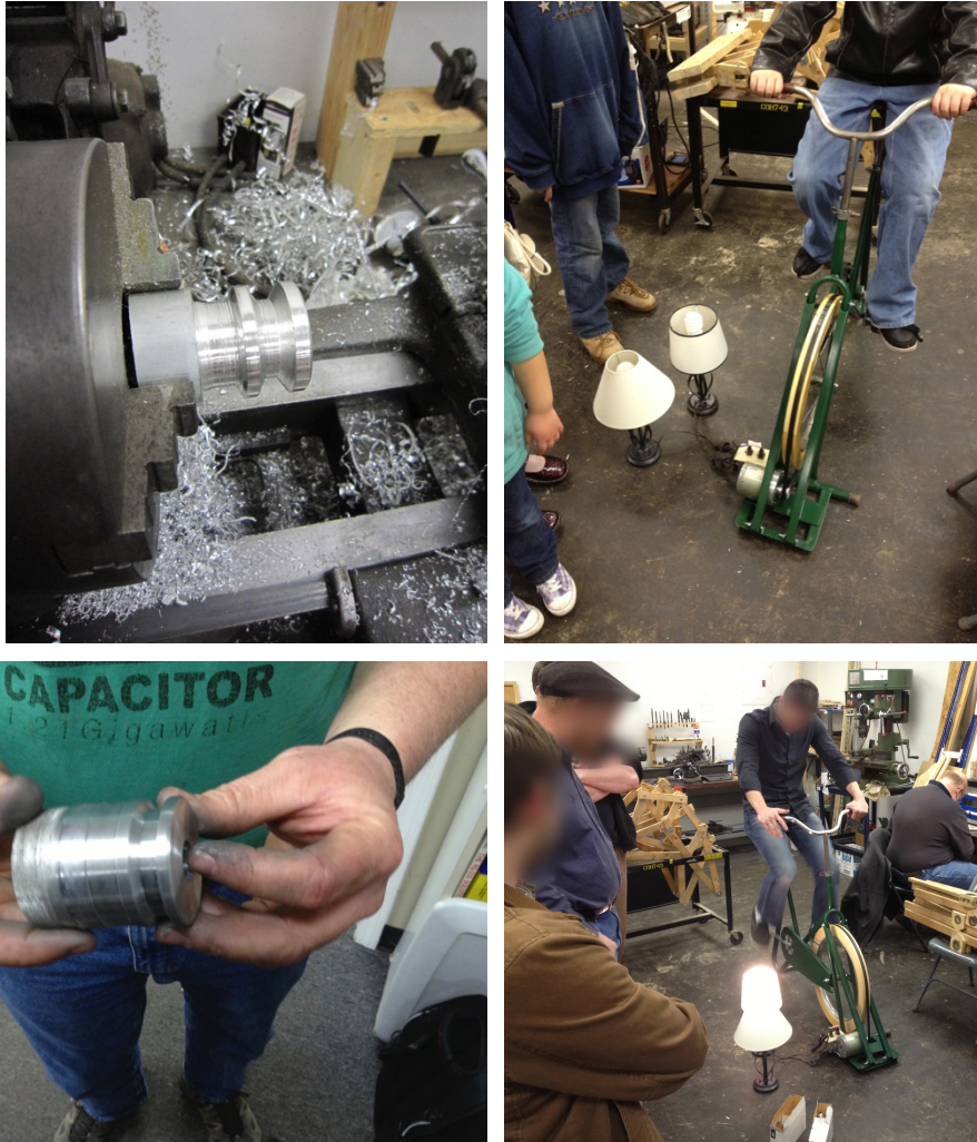
Figure 9. Bicycle generator and custom gear ratio.
