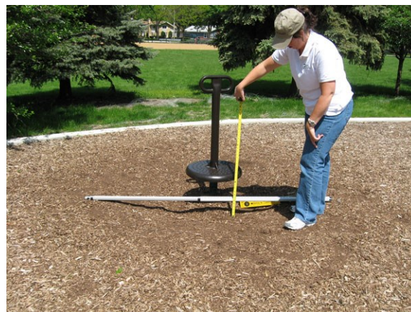
Photo 12: EWF with measurable displaced surface material at ground level play component.
