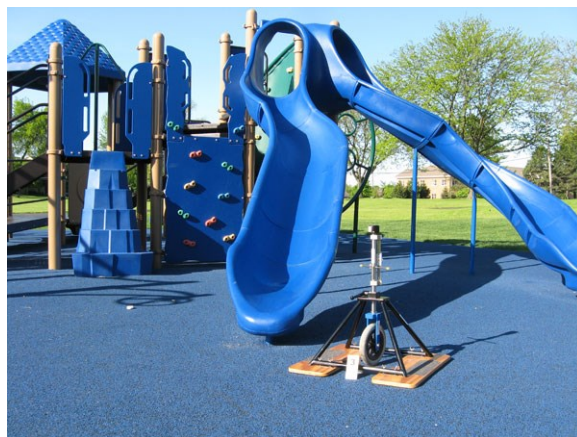
Photo 2: PIP with no recorded locations where the surface samples exceeded the accessibility standards.
