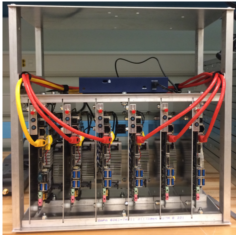
Figure 2. A LittleFe V4 frame showing six nodes exposed in a single, portable chassis, front view
