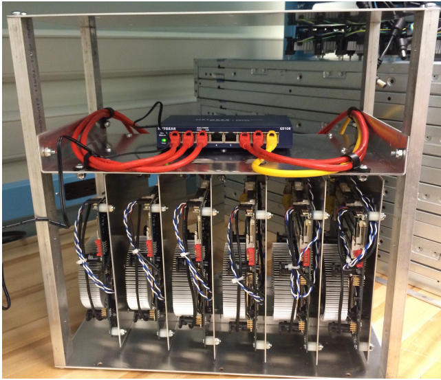
Figure 1. A LittleFe V4 frame showing six nodes exposed in a single, portable chassis, rear view.
