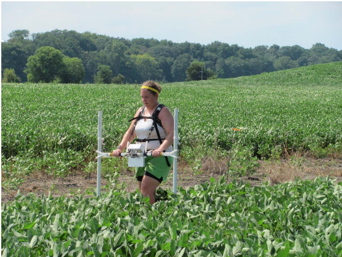
Figure 5.1. The author using the Bartington Dual Fluxgate gradiometer during the Summer 2011 magnetometry survey. Mound A is visible in the right side of the photo, Mound C is the gentle rise to the left.
