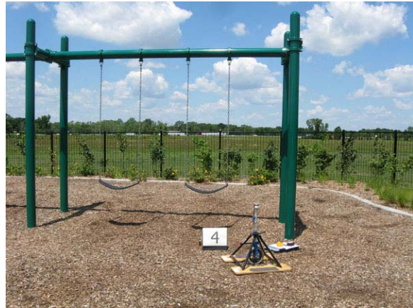
Photo 10: EWF with displaced area under swings.
