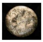
Antimony metal can be made to form a visibly onystalline structure by slowly cooling the motten antimony beneath a thick layer of slag. The antimony is reduced from stibnite (Sb2S3) by heating it with iron and saltpeter until fusion ensues. The antimony initially reduced must be further purified by repeated fusion with additional saltpeter before the star can be produced.
