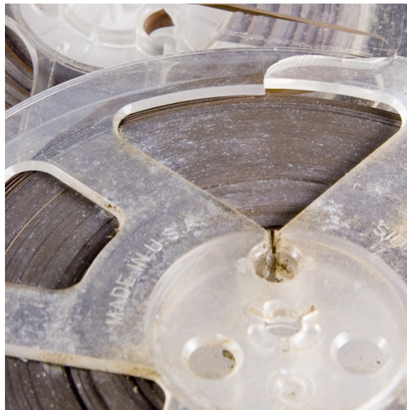
Figure 4: Open reel tape with severe fungus from the Bai T. Moore Collection
