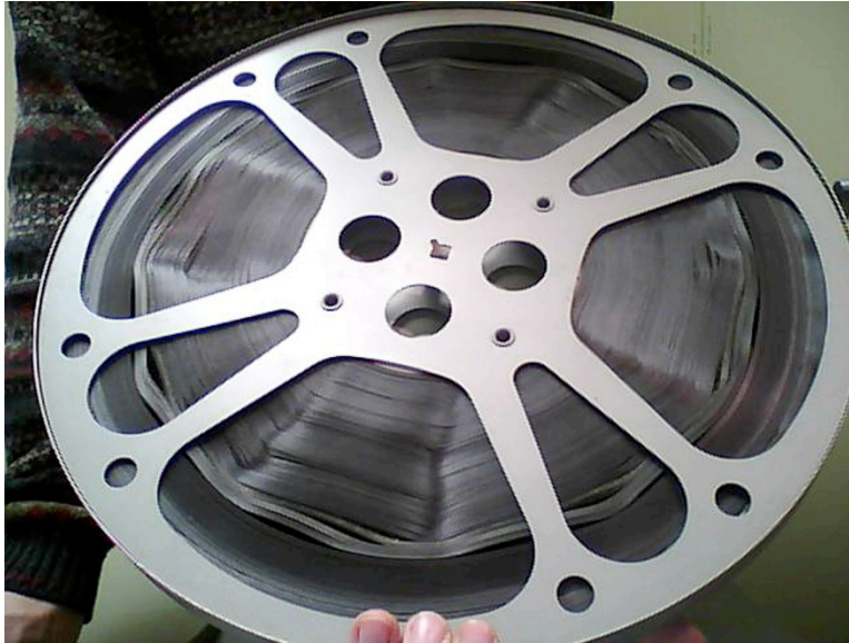
Figure 6: Film at the Glenn Black Laboratory of Archaeology with severe deterioration from vinegar syndrome.
