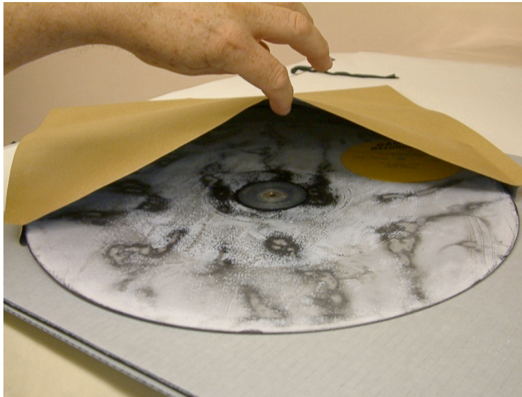
Figure 1: Lacquer disc at the Lilly Library exhibiting severe plasticizer exudation that is typical of the format. This is a recording of Orson Welles hosting the Jack Benny show in 1943.
