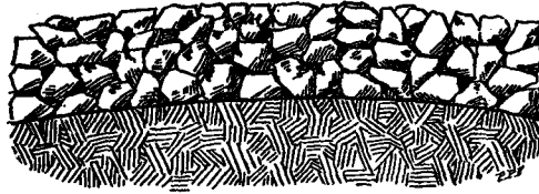
Fig. 19. First course of stone on a macadam road when partially rolled, showing how the roller packs it.
