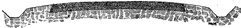
Fig. 14. Cross section of macadam road showing a compact foundation of earth supporting a solid and durable stone surface.
