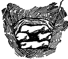
Fig. 11. Subdrain made of field stone for conveying spring water under or alongside of roads.
