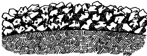
Fig. 18. First course of stone on a macadam road as it appears when spread ready for rolling.
